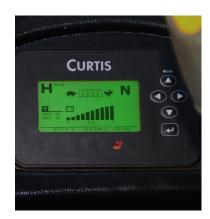
Multifunctional customizable LED panel with hour meter for accurate monitoring of charge level and timely maintenance.
