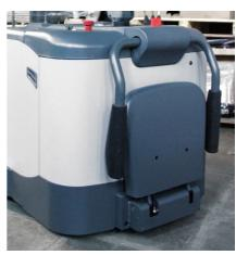
The platform as well as the handrails are integrated into the overall safety system and block movement when the operator is not on the platform
