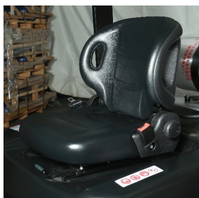
Built-in occupancy sensor in the seat will prevent the lift truck from moving without an operator.
