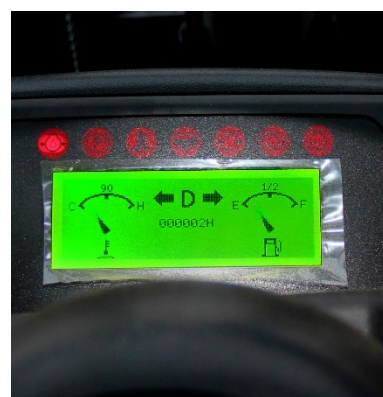
Multifunctional LED panel with hour meter to monitor timely maintenance.
