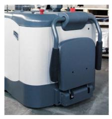
The platform as well as the handrails are integrated into the overall safety system and block movement when the operator is not on the platform
