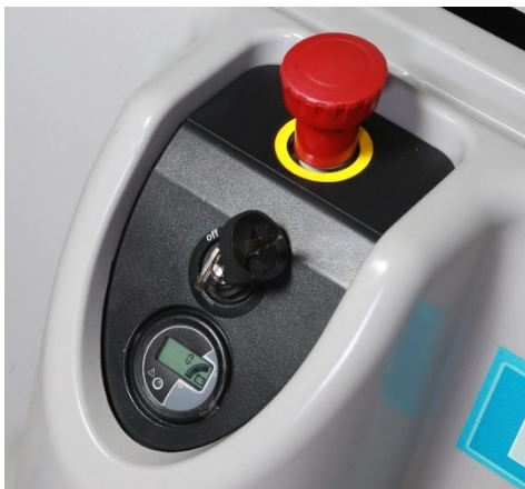
Emergency button, charge indicator and ignition key in the operator's field of view
