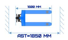
Minimum working corridor among electric pallet trucks Can work inside a truck
