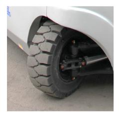
4 points of support with deep tread and reinforced lever, provide higher load capacity.
