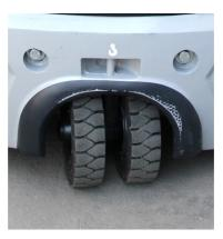
Increased steering angle of the twin rear wheels gives the loader maximum maneuverability.
